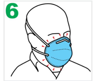
6 Perform fit check by ensuring seal of the mask. If air leaks upon exhale, adjust the mask.
